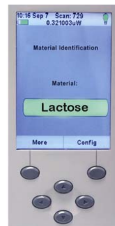
Typical raw material Identification result
